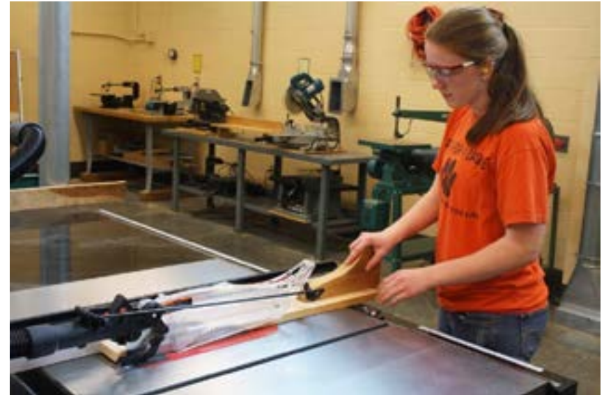
A high school senior in an upper level manufacturing class using a push stick to rip a piece of stock on a SawStop table saw.
